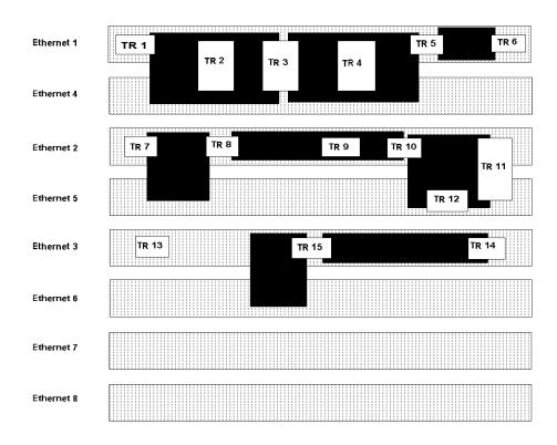
If Ethernet 1 is in use, any networks that overlap Ethernet 1 (meaning that they share the same backplane resources) are unavailable. As the diagram shows, using Ethernet 1 makes TR 1 through 6 unavailable.
